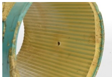
Figure 5. Connection can be viewed through translucent liner for easy reconnection after curing.
