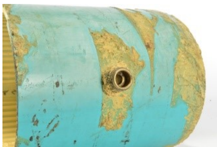
Figure 4. Poorly fitted connection is sealed by expanding grout.
